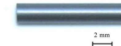
Fig. 4. Silicon-carbide sample used in the experiment (SiC, diameter 2.0 mm).
